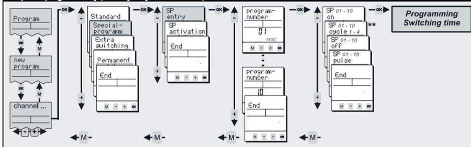
The yearly function of the switch is realised by special (weekly) programs which can be called up by date. Up to 10 special (weekly) programs can be entered (Program-Number 01 → Program-Number 10).
