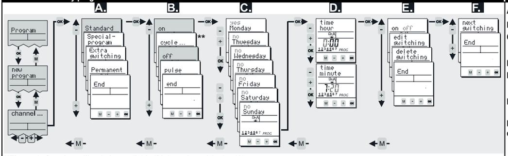
11. Example for the programming of STANDARD switching times (ON and OFF)
